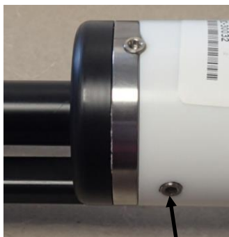
Cap screw securing battery / connector end cap (one each side)
