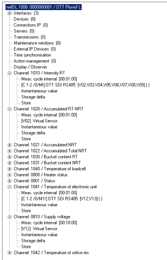
Fig. A4: Example configuration of an OTT DuoSens with 6 values recorded.
