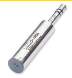
blue-green algae sensor submersible fluorometer Hydrolab based on the Turner Designs Cyclops-7
