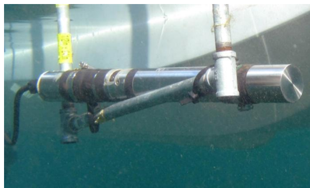
SUNA deployed for longitudinal profiling. Credit: Larry V. Korhnak
