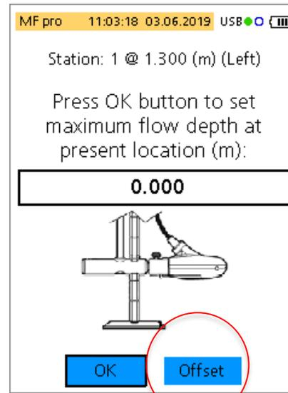
If the MF pro sensor is used with a rod which has a spike and the spike does not cave in the ground you'll need to enter the offset value. For OTT 20 mm universal rods it is 0.035 m. The offset can be changed at each station.
