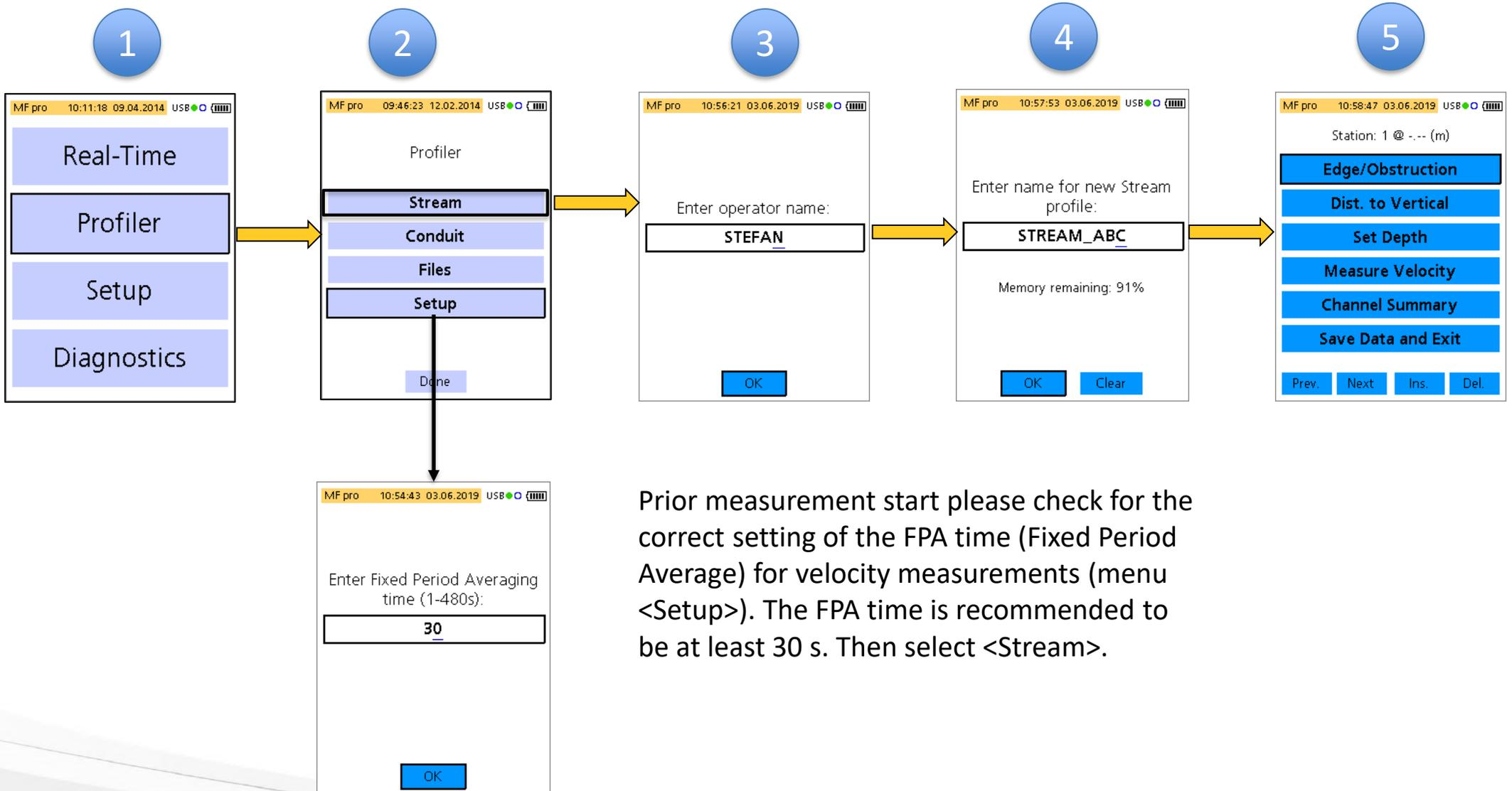
Prior measurement start please check for the correct setting of the FPA time (Fixed Period Average) for velocity measurements (menu <Setup>). The FPA time is recommended to be at least 30 s. Then select <Stream>.
