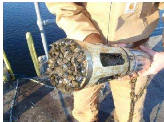
Above: Jeremy Brill and Craig Just of IIHR with their sensors Below: The DS5X covered in mussels and sediment after extended deployment
