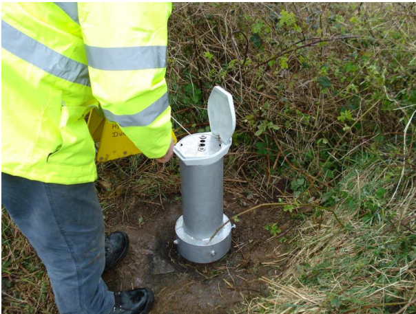
Bog of the Ring monitoring site: Two OTT Orpheus Mini's installed in the well at different depths and OTT KL 010 Contact Gauge used for conducting as reference measurement. (Photo courtesy of M. Browne, Ireland EPA)
