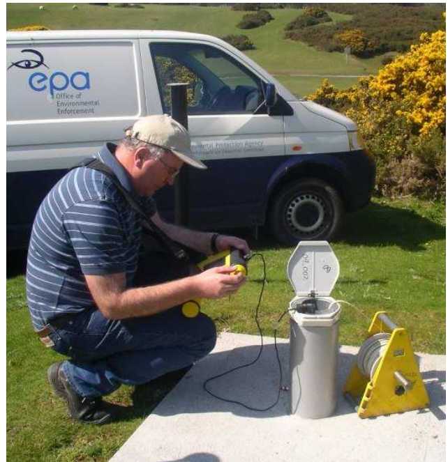
WFD groundwater monitoring site: OTT Orpheus Mini installed in the well and OTT KL 010 Contact Gauge for on-site reference measurement. (Photo courtesy of M.Browne, Ireland EPA)
