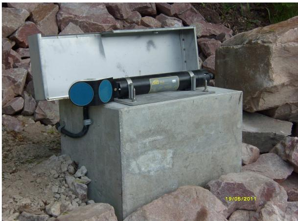
Mounted sensor of the upper measuring path with lockable protection cover.
