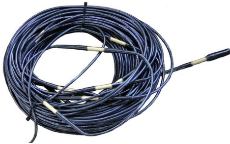
Measurement chain with 16 temperature sensors
