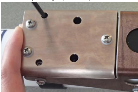
Push copper anti-foulant assembly while tightening captured cap screws
