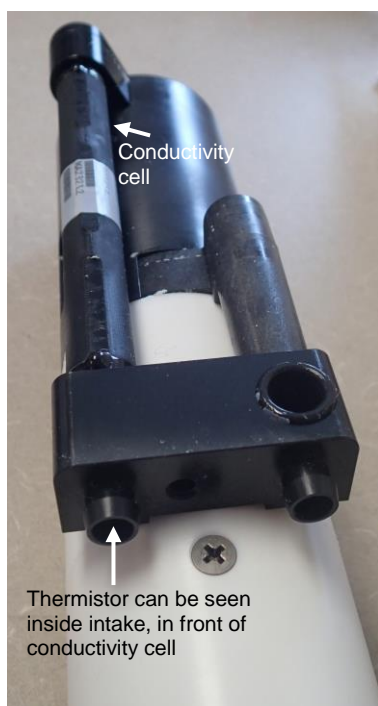
Shown with conductivity cell guard and anti-foul fittings removed
