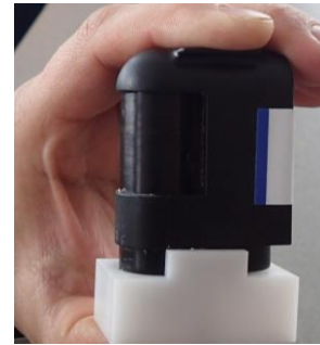
pH sensor and cap (filled with KCl solution to keep glass bulb and reference electrode from drying)
