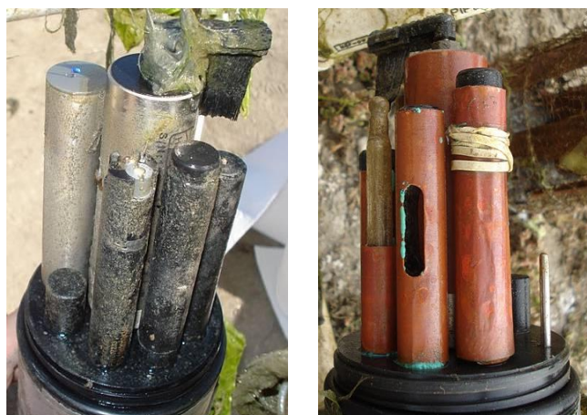
Above: sensors fouled after deployment (l) vs. sensors deployed with copper tape (r)
