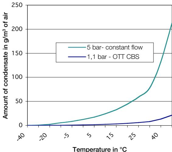
Diagram 1: Condensate at 60 % relative humidity per m<sup>3</sup>
