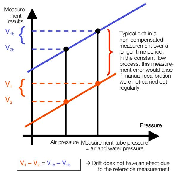
Figure 4: OTT CBS Drift-free Measurement Principle
