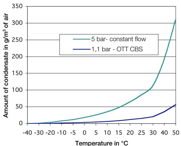
Diagram 2: Condensate at 80 % relative humidity per m<sup>3</sup>
