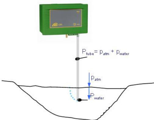
Figure 3: Determination of water level
