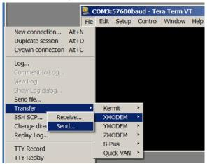
**10.** Select the downloaded firmware in the new window and push **Open**. The firmware is sent to the sensor.
