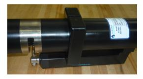
SUNA optical area pointed sideways, and down, to reduce the collection of sediment and bio-fouling.
