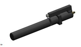
The wiper drive shaft has a mechanism that lets the wiper be moved manually without damage. Make sure that the wiper is not bent or pushed off of its axis of rotation.
