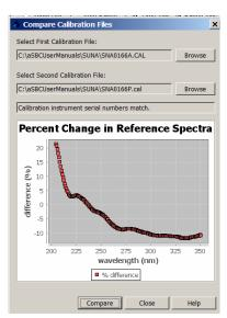
A typical update interval of 3–6 months with no more than 100 hours of lamp use should cause a change of no more than 10% in the 215–240 nm interval.
