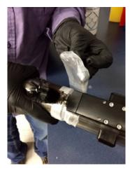
5. Break a small hole in the top of the Parafilm<sup>®</sup> and fill the optical area with DI water.
