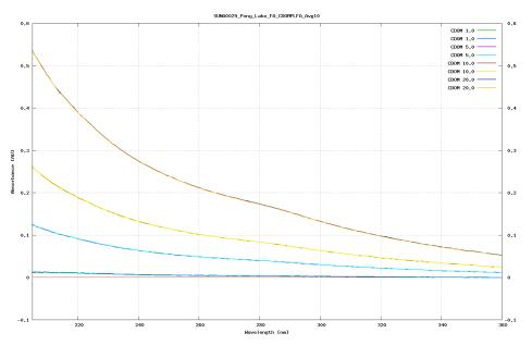
The model to calculate nitrate fits for 4 parameters: nitrate, bromide, a temperature coefficient and a linear baseline correction that accounts for all additional absorbing species. If the absorption of the sample is high (default cut-off = 1.3 AU), the model can no longer be used effectively to fit parameters or calculate nitrate concentration. The SUNA V2 data output is a root mean square error parameter that indicates the quality of the fit of the models to the absorption curves.
