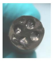
Lubricant on socket end of the connector
