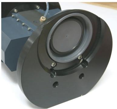
9. Install the retaining ring with the new filter into the base of the sensor. Tighten by hand until the retainer stops firmly ("bottomed out"). To make sure the assembly is "bottomed out," use the rectangular tool to tighten the assembly no more than 1/8 of a turn past hand-tight.
