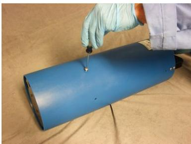
5. Hold the bottom of the sensor and put it vertical to slide the protective sleeve off.
