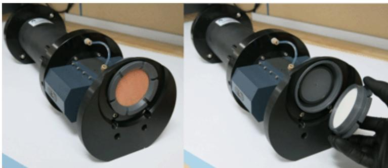
3. Use the rectangular tool supplied by the manufacturer to loosen the retainer disk if the retainer is difficult to remove.
