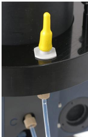
20. Lubricate the bulkhead connectors.
