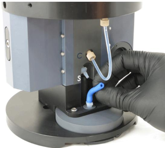
6. Disconnect the syringe and pinch the tubing so that the cleaning solution stays in the tubing.
