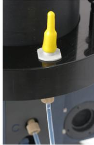
5. Install new cartridges. Refer to the section on [Assemble the sensor](#) on page 9 for details on this procedure.
