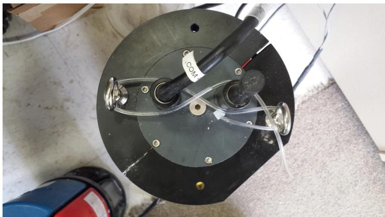
5. Put the sensor on its side, hold the eye bolts, and align the screw holes for the sensor and the protective sleeve.
