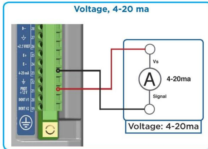
The key settings for 4-20mA sensors connected to the 4-20mA input are:
