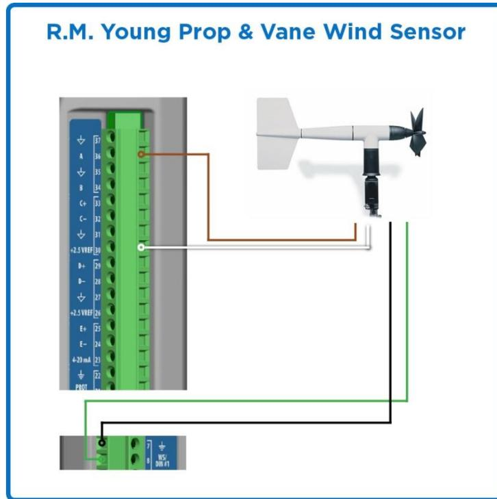
\* A 1.0 MOhm resistor needs to be placed from VREF (or SIGNAL GROUND) to AZ SIG. This ensures that the value always goes to 355 (or 0 with SIGNAL GROUND) when the potentiometer is in the open region.
