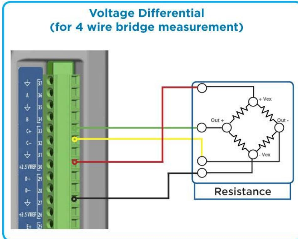
The key settings for strain gauge sensors are:
