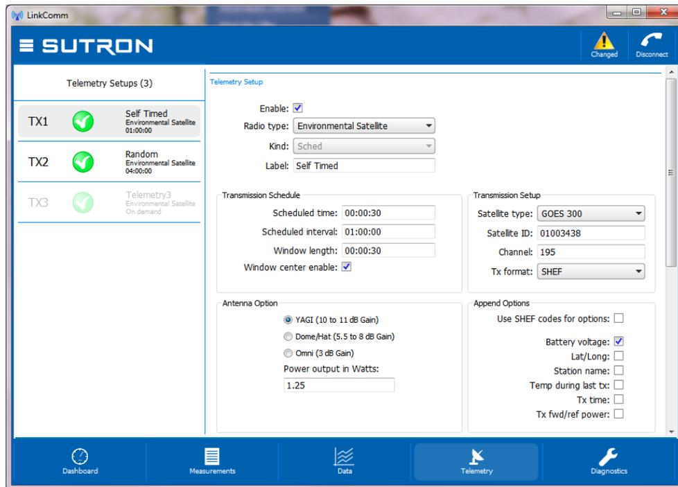
The column on the left shows that multiple setups are possible with the satellite -- one for scheduled transmissions, one for random transmissions and one for on-demand transmissions. Each is configured and enabled separately. If none of the telemetry setups are enabled, the system will show an error if on the dashboard.
