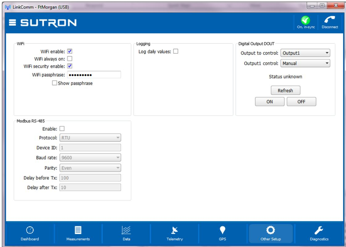
The controls in the **Digital Output DOUT** section can be used to view the status of the digital output, and to control its state. Press the **Refresh** button to display the current state of DOUT.
