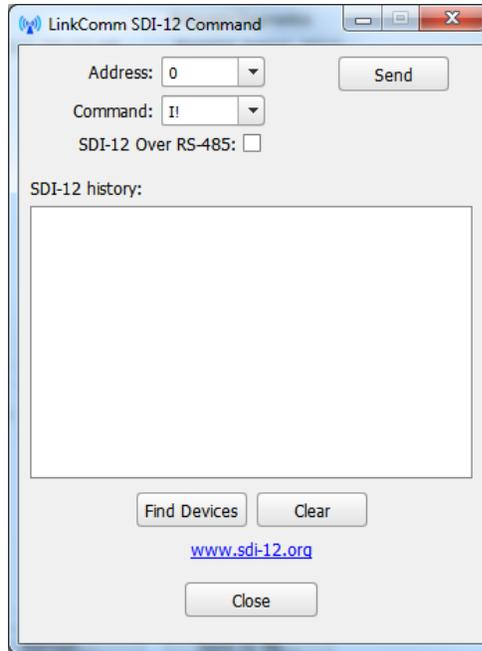
To send a command to an SDI-12 device connected to Satlink, enter the **Address** and **Command** fields, and then press the **Send** button. Be sure to check **SDI-12 over RS-485**, if you need to send the command over the RS-485 bus. The results of the command are shown in the SDI-12 history window.
