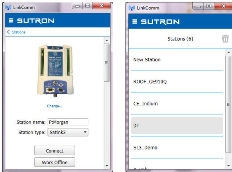
To work with the selected station, press “Connect”. The software will use connection settings (USB, RS232, WiFi) and try to communicate with the site.
