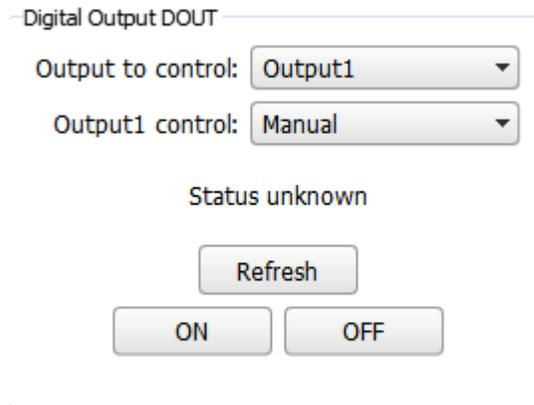
LinkComm allows setting either or both outputs to be turned on/off based on the Output control. The output control has the settings for each output.
