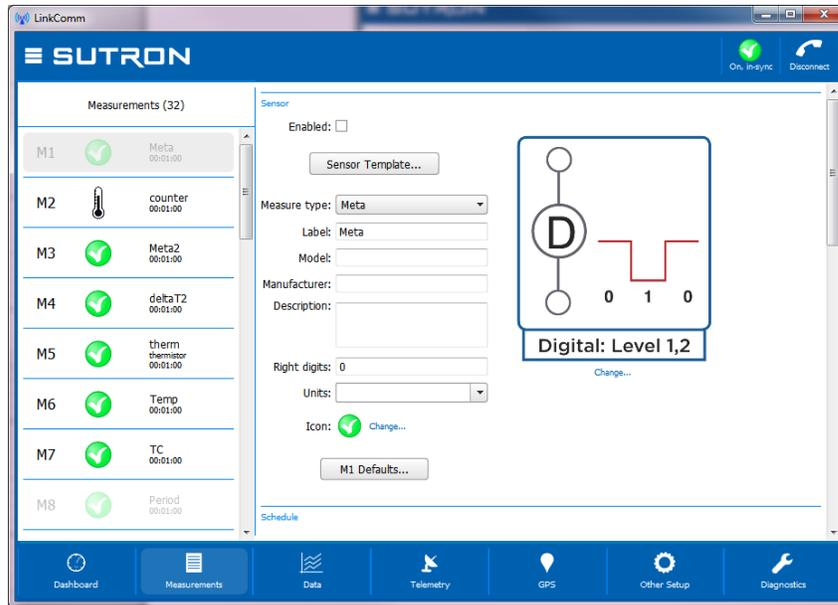
The left side of the measurements tab shows a list of all possible measurements. The right side of the measurements tab shows the details of the selected measurement. The details are the settings used to determine how the measurement is taken and how the data is processed by the system. The settings include schedule, Configuration (including wiring diagram), Processing, Alarms, Logging, Tx Content.
