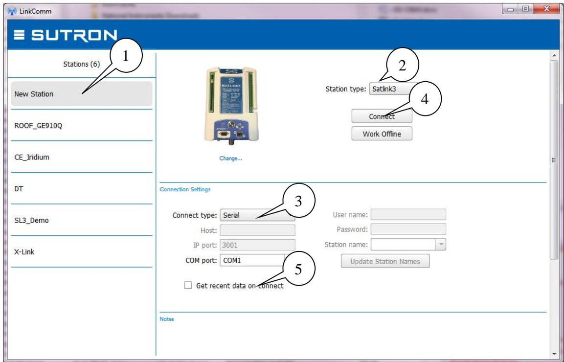
You can also set the software to get recent data (5). “Get recent data on connect”, when checked, will cause LinkComm to download the last week of data for display in a graph on the dashboard tab, every time you connect to Satlink. This can be a considerable amount of data (several k-bytes). Here again, you may choose to disable this feature to reduce data costs.
