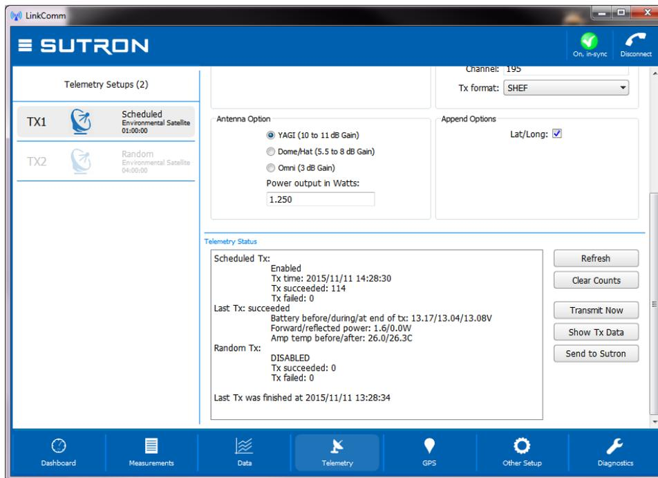
The status text is retrieved from Satlink the first time you display the telemetry tab, and can be refreshed as needed on demand.
