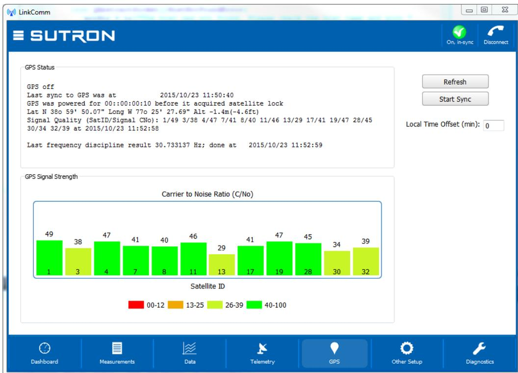
In order to give the user a better idea of the quality of the GPS signal, Satlink Logger provides messages that indicate how long the GPS module was powered before a time sync was initiated. If the last GPS sync was a part of a transmission, this number should roughly be equal to the GPS acquire time. If the last sync was user initiated, then this number will indicate how long it took the GPS module to acquire the signal necessary to provide an accurate time.
