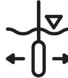
Remotely monitor probe movement in the field with an internal inclinometer, enabling warnings if sensor position has changed due to in-stream events via automatic status flags or direct measurement.
