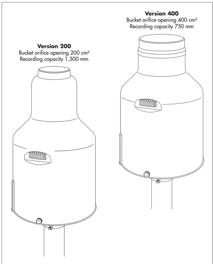
Every 6 seconds, the precipitation gauge determines the weight of the collecting bucket including its content using a resolution of 0.001 mm (= raw data). The difference between this measured value and the weight of the empty collecting bucket gives the current bucket content.
