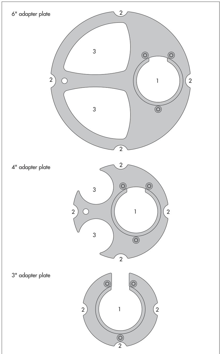
Fig. 7: Accessories for installation – Part 2
