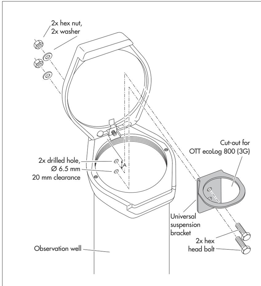
Fig. 13: Installing the OTT ecoLog 800 (3G) into observation wells of 3" diameter and above with a top cap without cut-out.
