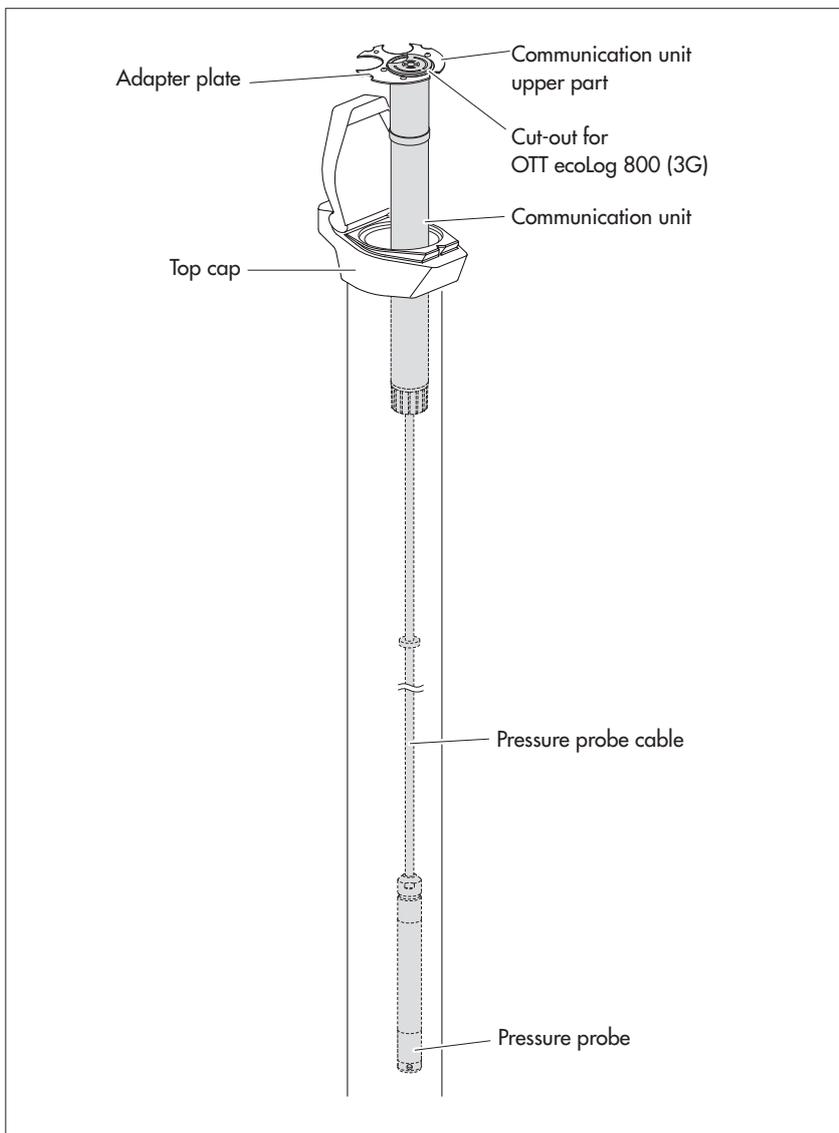
Fig. 11: Installing the OTT ecoLog 800 (3G) into a 3", 4" or 6" observation well.
