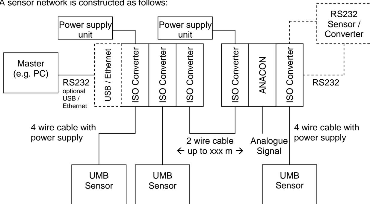
**Master:** The master is connected to the RS232 interface built into the ISO converter. An interface module for USB and Ethernet via virtual COM port is also available as an option.
