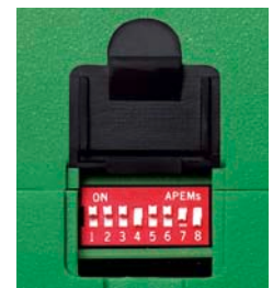
DIP switches for easy programming
