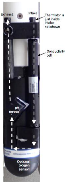
Figure 2: HydroCAT-EP Flowpath
