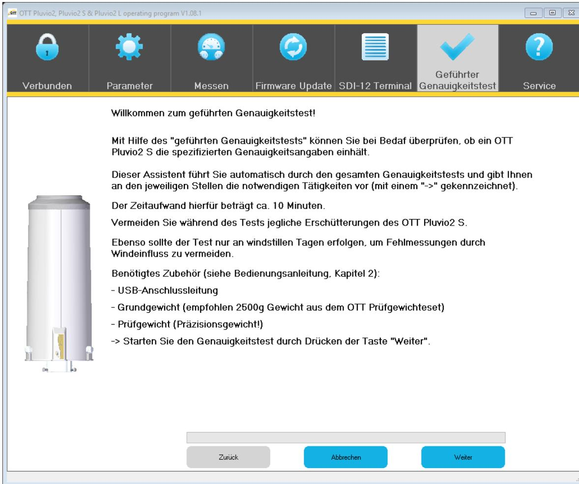
The screenshot shows the 'Geführter Genauigkeitstest' (Guided Accuracy Test) screen in the OTT software. The window title is 'OTT Pluvio2, Pluvio2 S & Pluvio2 L operating program V1.08.1'. The navigation bar at the top includes icons for 'Verbunden', 'Parameter', 'Messen', 'Firmware Update', 'SDI-12 Terminal', 'Geführter Genauigkeitstest' (highlighted with a checkmark), and 'Service'. The main content area contains the following text:
