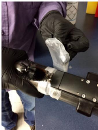
5. Break a small hole in the top of the Parafilm® and fill the optical area with DI water.
