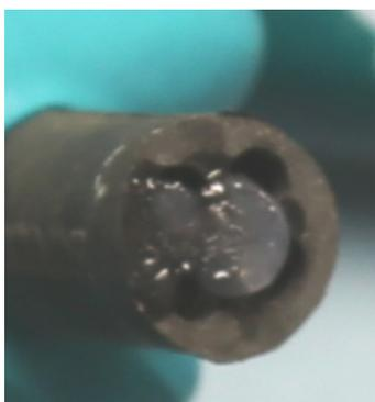
Lubricant on socket end of the connector
