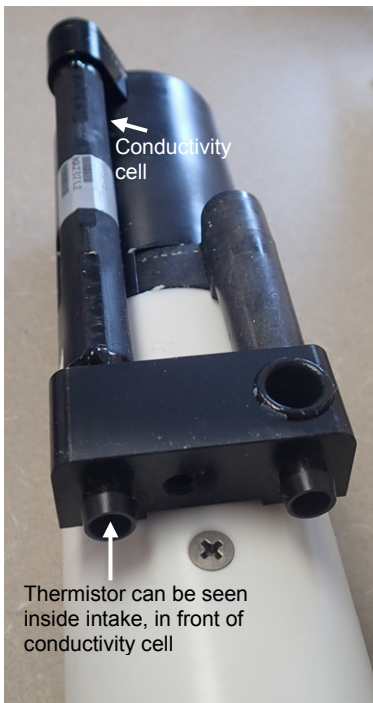
Shown with conductivity cell guard and anti-foul fittings removed
