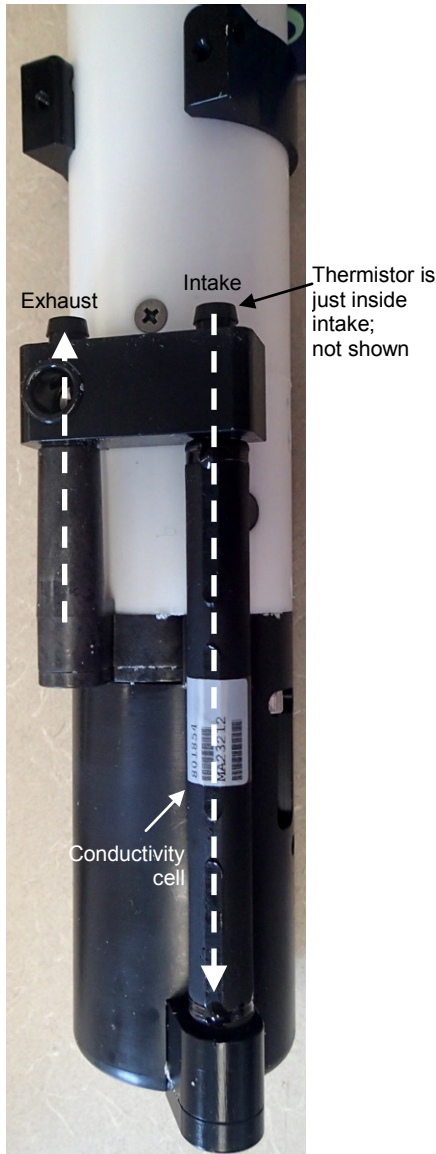
Shown with conductivity cell guard and anti-foulant fittings removed
