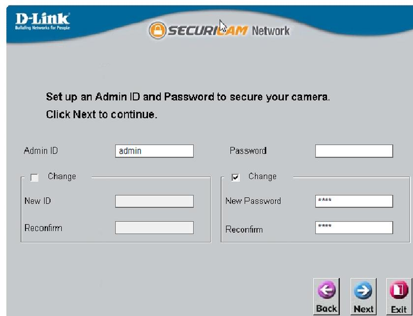
The screenshot shows the same D-Link Securicam Network setup interface as the previous one. The title bar and heading are identical. In this version, the "Change" checkbox under the Password field is checked. The "New Password" and "Reconfirm" text boxes in the sub-section below it contain four asterisks (\*\*\*\*). The "Back", "Next", and "Exit" buttons are still present at the bottom right.
