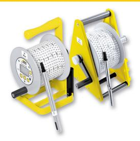
OTT Contact Gauges for measurements of depth to water, temperature and conductivity
