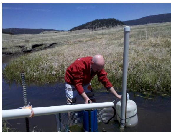
Figure 4. Photo showing Dr. Corey Koch helping to deploy the Cycle-PO4 in the Jemez. Relationship between two months of continuous data from a Cycle-PO4 and Jemez river discharge (USGS Gage 08324000, downstream; cubic feet per second (CFS)).
