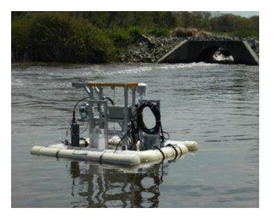
**Figure 1**. Sea-Bird Coastal / Hach Hydromet Foreman Branch Nutrient and Water Quality monitoring platform located on Chino Farms.
