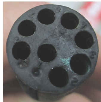
Damaged socket face
