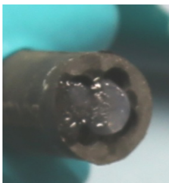
Lubricant on socket end of the connector
