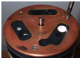
Figure 5 Copper faceplate attached to optical face
