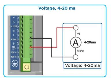
The key settings for 4-20mA sensors connected to the 4-20mA input are:
