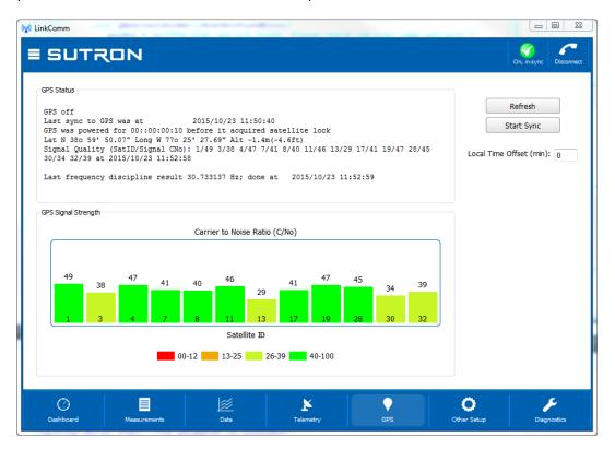
In order to give the user a better idea of the quality of the GPS signal, Satlink Logger provides messages that indicate how long the GPS module was powered before a time sync was initiated. If the last GPS sync was a part of a transmission, this number should roughly be equal to the GPS acquire time. If the last sync was user initiated, then this number will indicate how long it took the GPS module to acquire the signal necessary to provide an accurate time.
