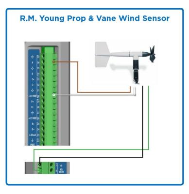
\* A 1.0 MOhm resistor needs to be placed from VREF (or SIGNAL GROUND) to AZ SIG. This ensures that the value always goes to 355 (or 0 with SIGNAL GROUND) when the potentiometer is in the open region.
