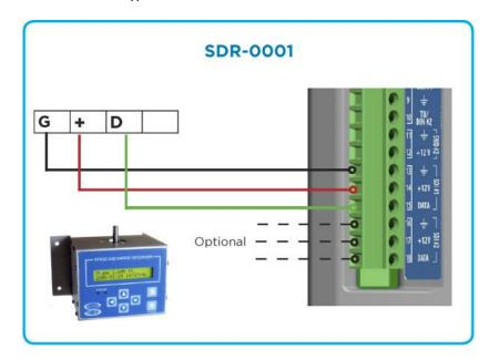
The figure below shows the typical SDI-12 sensor connections.
